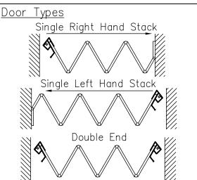
Door Types: Single or Double End only - no Pairs Single End *must* specify left or right hand.
