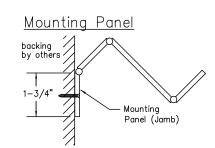
Direction of mounting panel (jamb) varies based on door construction. Consult factory for specific information.
