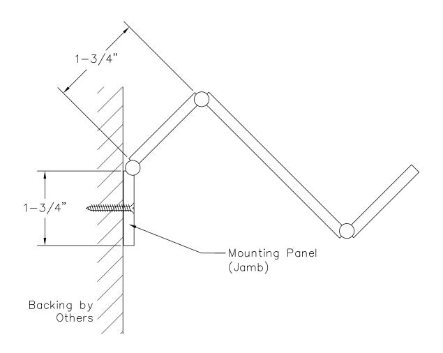
Direction of mounting panel (jamb) varies based on door construction.
