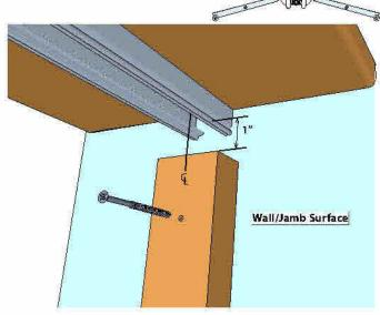
Push the door over the post. The post will snugly fit between the mounting panel flaps. Screw the mounting panel flaps to the post using the provided  $\#6 \times 1\frac{1}{2}$  flat head screws. Place a screw about 6" from the top and bottom of the post and 2 additional screws equal distances between the first 2 screws. Repeat anchoring the 2nd flap being sure to slightly offset the screws so they won't meet in the middle of the post.
