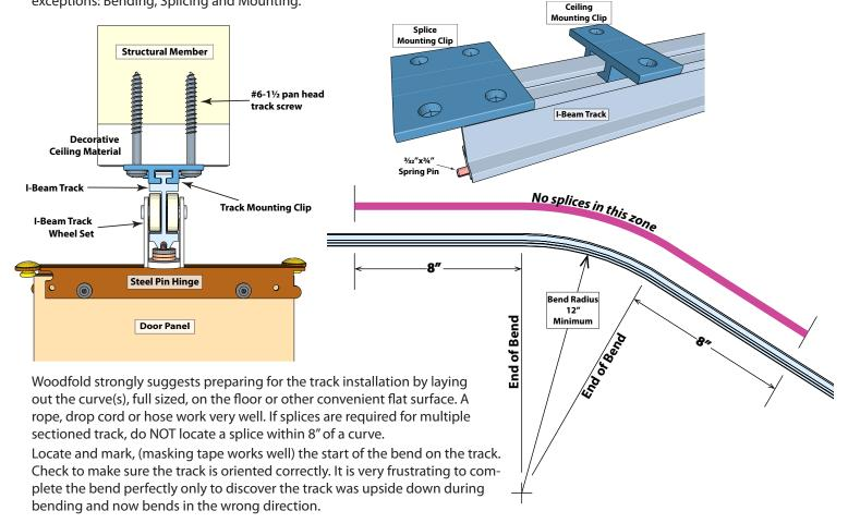
Place the track around a sturdy round object with the track contacting the object just on the bend side of the masking tape mark. Now pull gently on the tail to bend the track.
